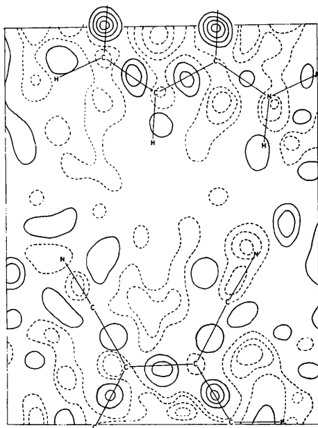
Fig. 4. The difference Fourier map through the plane ( \bar{1}12 ). Solid contours show positive density at intervals of 0.05 \text{ e \AA}^{-3} , starting with 0.05 \text{ e \AA}^{-3} . Broken contours show negative density at the same intervals, starting with -0.05 \text{ e \AA}^{-3} .
